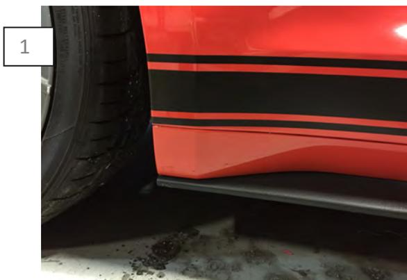
Wash the fender and rocker pannel with soap and water. Allow the panel to dry. **\*\*Recommended:** Wipe the panel down with isopropyl alcohol to ensure the cleanest surface possible.
