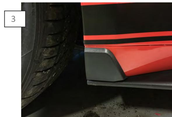
Remove the 3M tape backing, install the winglet onto the fender. Apply firm even pressure to ensure proper adhesion.
